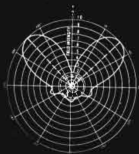
Typical measured Pattern #21 Peak hor. power gain 3.38
